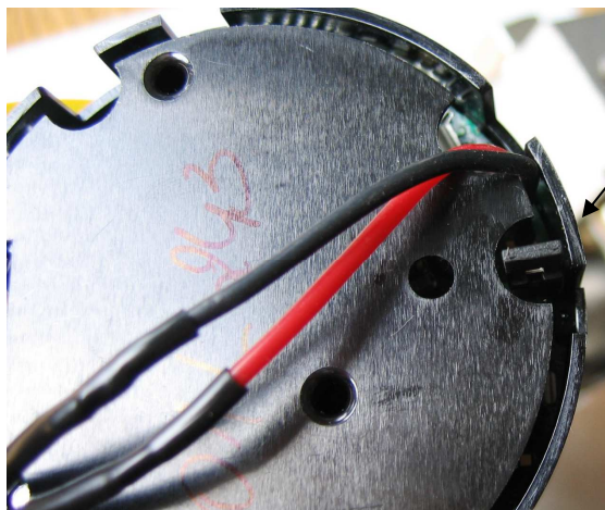
Fig. 5. View of the back lighting jumper on transmitter electronics board for PYRP... , PYRD... in Exd versions (unit display from rear).
