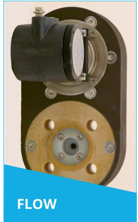
Each instrument can be provided with one of seven standard orifice ratios which enables a wide range of flow rates to be accommodated. When using fluids other than fresh water these values will of course alter. It should be also noted that the head loss values are those occurring immediately across the orifice and that up to 50% of this head loss can be recovered by providing at least ten diameters of straight plain pipe either side of the flow switch.
